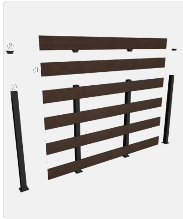
③ Fence Board TH-05D(140x13mm)
